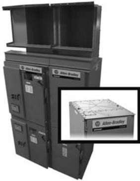
The Allen-Bradley CENTERLINE ArcShield arc-resistant controller provides rugged process control for applications requiring a higher level of personnel protection. ArcShield products are compliant to the IEEE C37.20.7 standard, and provide Type 2 protection during an arc flash.
