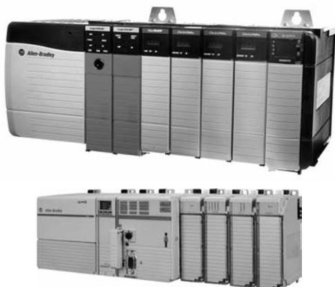
A GuardLogix® controller is a full-function Logix processor that also provides safety control. The GuardLogix system is a dual processor solution that uses a primary controller and a safety partner to achieve SIL 3, PL e. A major benefit of this system is that it is a single project, with safety and standard control together. The GuardLogix system is a 1oo2 safety architecture that provides unmatched safety and ease of use.
